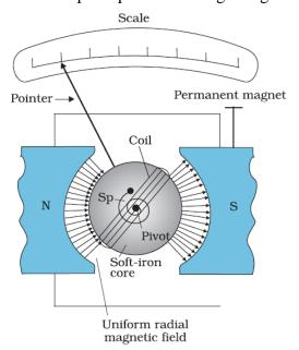
The galvanometer consists of a coil, with many turns, free to rotate about a fixed axis .the coil is placed in a uniform radial magnetic field. There is a cylindrical soft iron core which not only
